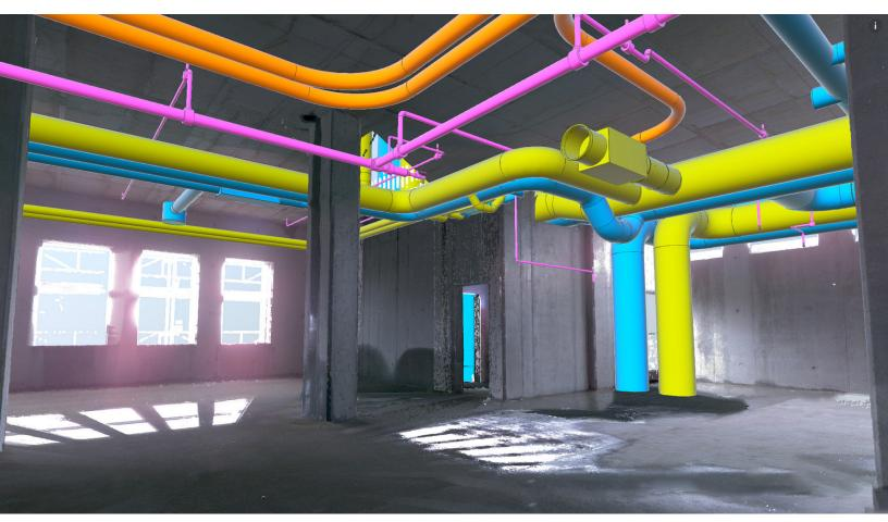
Imerso's scanners capture the as-built status throughout the construction phase with point clouds – a collection of 3D data points that accurately digitize real-life physical spaces, such as a building, a floor, or a room
